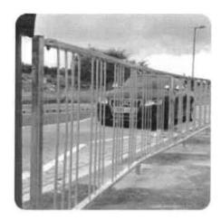
Pedestrian guard rail typically costs around £3,000 which would cover a 10m length.
