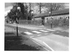
Divided zebra crossing (including high friction surfacing on approaches if required) typically costs between £25,000-£35,000.
